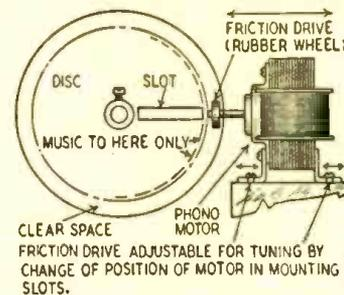
Fig. 1—End view showing slot and rim drive.
