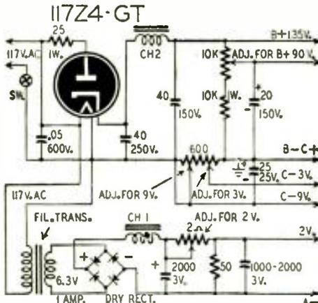
ALL FINAL VOLTAGE ADJ. MUST BE MADE AT FULL LOAD
