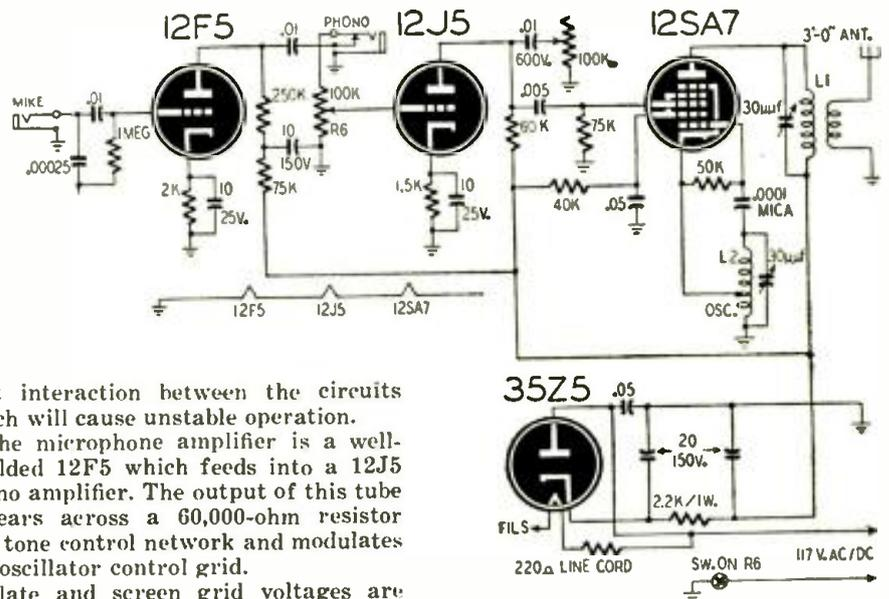
vent interaction between the circuits which will cause unstable operation.
