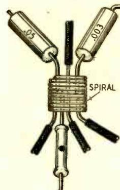
springlike spiral about 1/4 inch long. The diameter will depend on the number of wires to be joined. Leads from the components may be inserted into either or both ends and solder flowed into the spiral. This makes a good electrical connection that is mechanically strong.
