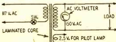
One of these transformers should have core-type laminations; the other a shell-type core. Remove the secondaries from the one with the shell-type core, then carefully unwind the primary. Remove the secondaries from the transformer with the core-type laminations and in their place rewind the primary from the other transformer. In some case a winding may be found which can be slipped on the core leg "as is".
