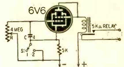
open. When the switch is thrown to position No. 2, the cathode resistor is shorted to permit the charge to leak off the condenser through the variable resistor. The relay closes when the plate current has risen to the proper value.
