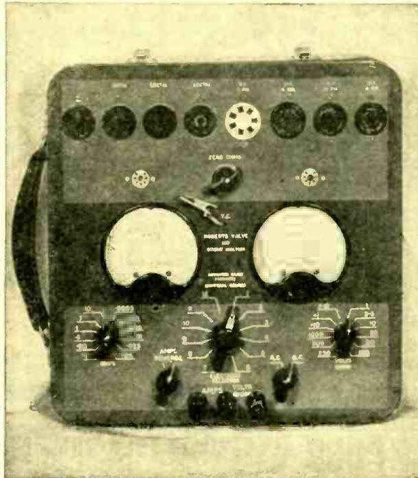
Test Tubes for Current, any electrode, A/C & D/C, 11 ranges 0- 2.5 amps.
