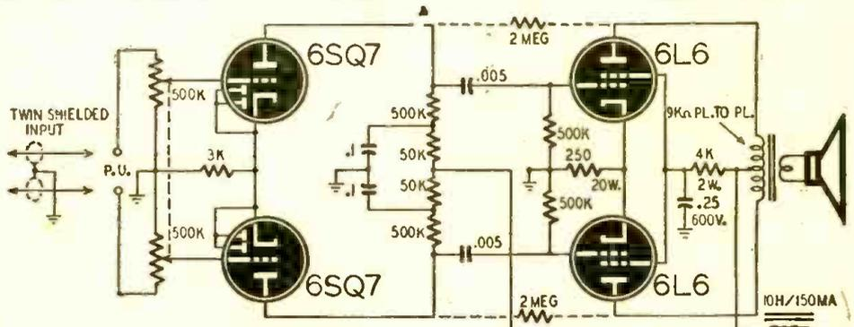
2-conductor shielded cable. The conductors are connected to the high sides of the ganged volume controls and the shield is grounded. If desired, inverse feedback may be used by connecting two 2-megohm resistors as shown by the dotted lines.
