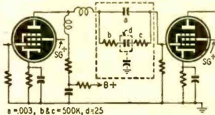
A typical coupling network is shown within the box in the first figure. It is composed of an R-C network in which the stray and distributed capacitance to ground must be kept low to avoid resonance effects and power loss. Typical component values are shown.
