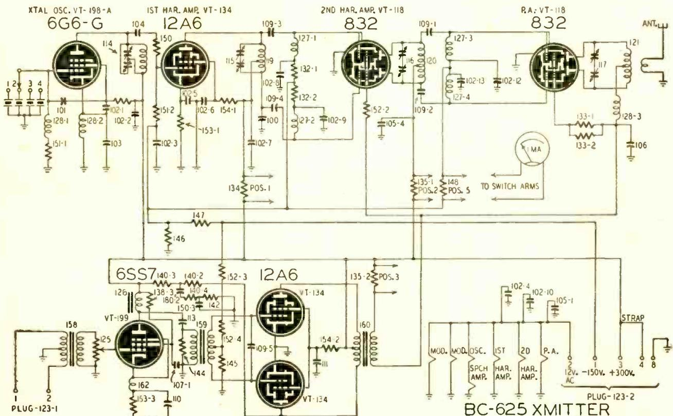
Complete schematic of the converted BC-625. Very little work was necessary to make this an excellent transmitter on the 144-mc band.
