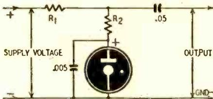
as an a.f. oscillator whose frequency may be controlled by plate voltage or the value of R1 plus R2. The output voltage is determined by the ratio of R1 to R2. The table gives the values of R1 plus R2 to give a 400-cycle note for different supply voltages.
