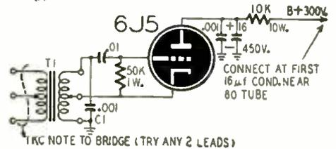
Here is a circuit of an oscillator that may be used as a source of 1,000-cycle current. The value of C1 will determine the frequency of the tone. If the inductance of T1 is 25 henries, the oscillator will tune to the required frequency with a 0.001- $\mu$ f condenser for C1.
