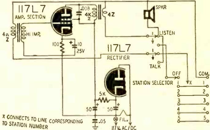
Fig. 4—A simple system which uses 1 tube at each end of the circuit.
