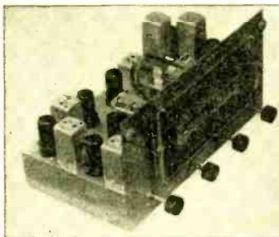
The dimensions of the tuner exclusive of power supply are; height 7 3/8", width 13 1/2", depth 9 inches. The power supply is a small separate unit.—RADIO-CRAFT
